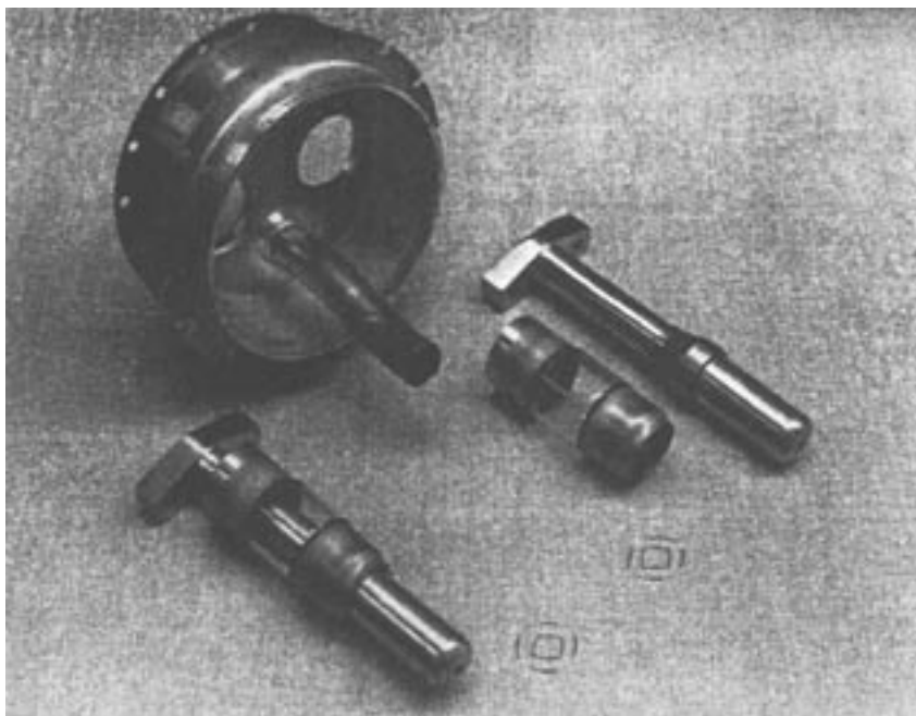
Components of a power triode header assembly, by English Electric Valve Co Limited, together with the inserts of Pallabrazz S10 wire that are used in the brazing operation. Brazing is carried out induction hearing, and brazing time is about thirty seconds.
