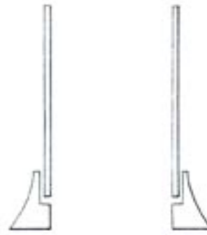
Fig. 1 Simple tube-to-fitting joint used for the costing exercise
